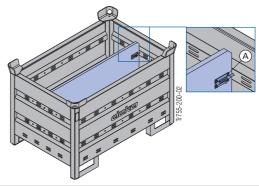
A Slide-bolt for fixing the partition
